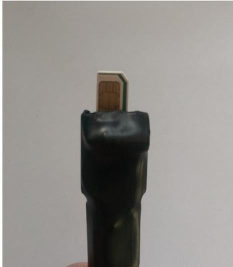
With the white sticky foam facing away from you ensure the SIM card has the contacts facing you and the cut corner to the top right. When removing or inserting the SIM ensure that power is removed from the module. The module has a network connection when the LED near the SIM slot flashes every 2-3 secs. Every 1 sec indicates no network connection.
